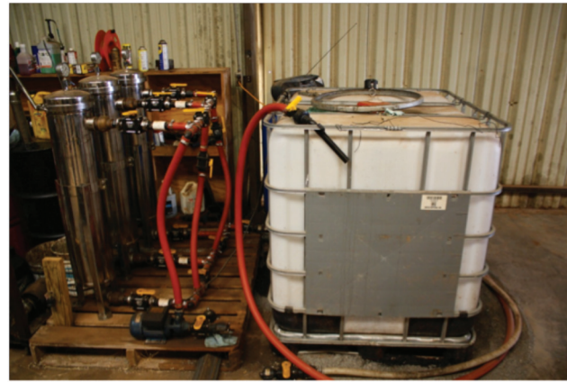
Figure 2: On-farm biodiesel filtration system.
