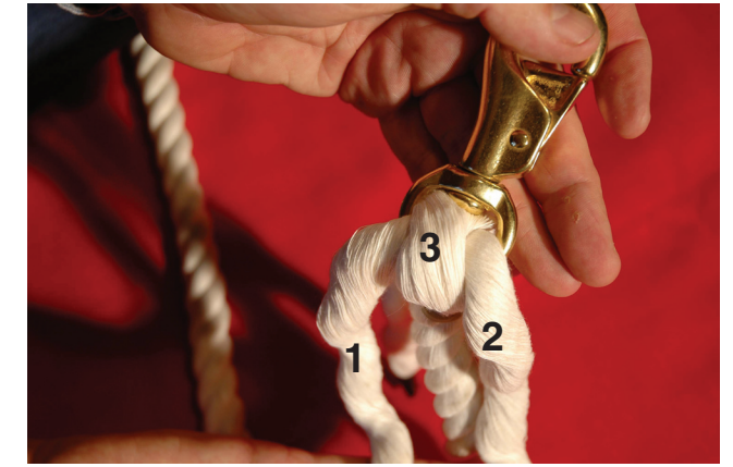
4. The third strand will run over the initial two strands. Pull the strands tight. You will then begin the back plaiting process.
