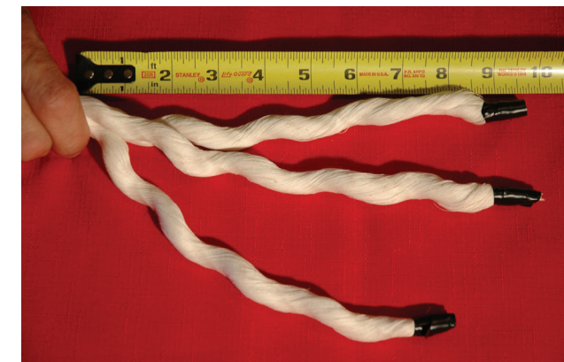
1. Unravel about 8 to 10 inches of rope, and tape off ends to keep the strands from fraying.
