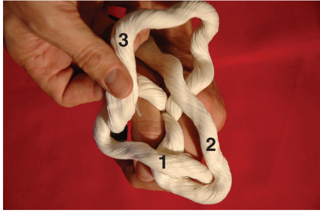
5. Place the tail of the third strand (3) over the tail of the second strand, and into the loop formed from the first strand.
