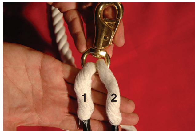
2. Place two of the unbraided strands through the eye of the snap.
