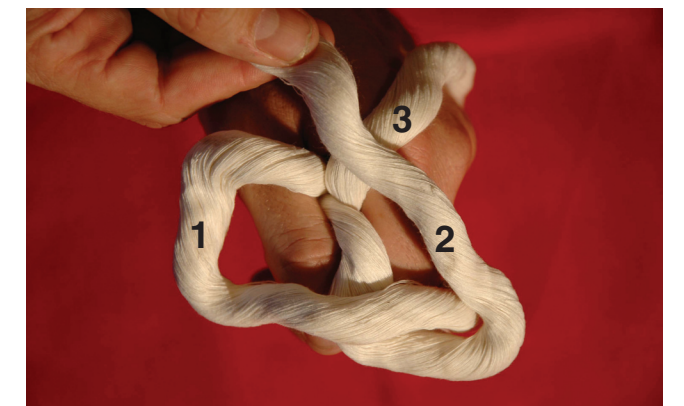
4. Place the adjacent strand (2) over the tail of the first strand and third strands.
