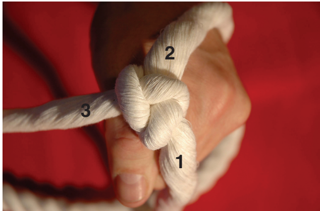
7. Pull the crown knot tight. Back braiding relies on this knot to be even and secure. The following steps involve braiding the loose strands (tails) into the unraveled portion of the rope beneath the crown knot.
