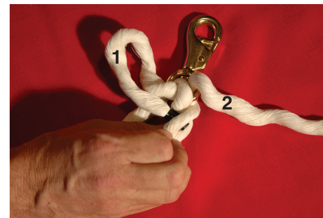
5. Begin with one of the two initial tails. Move over one strand to its right and then under the next strand.
