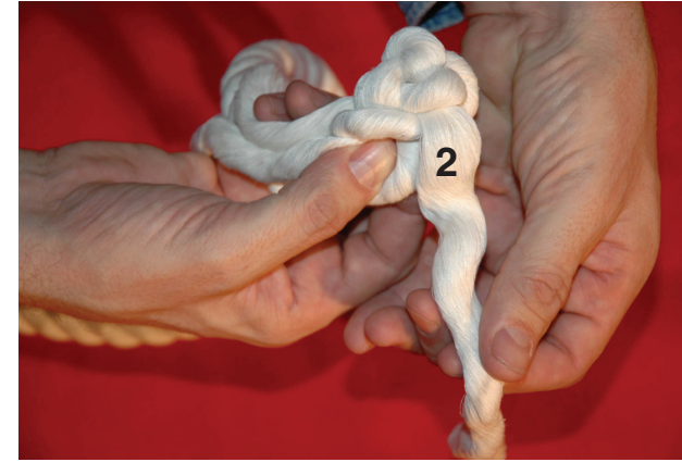
11. Moving to the right, grasp the next unraveled strand from the crown knot and repeat the process.
