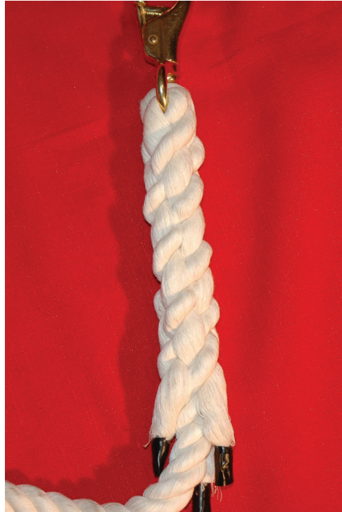
8. When completed, the snap is secured in place with 8 to 10 inches of back plaiting. Similar to the handler's end of the rope, the loose tails can be cut even with the plaits. If the plaits are not tight, tape can be used to encircle the rope in the location of the cut tails.
