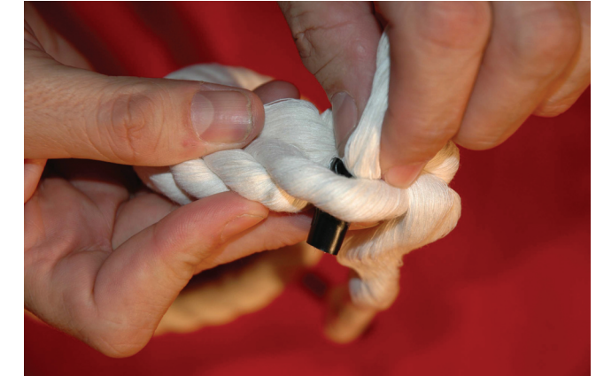
12. Place the tail over one, then under the next unraveled strand. Pull it tight, and complete the same process with the remaining (third) strand.
