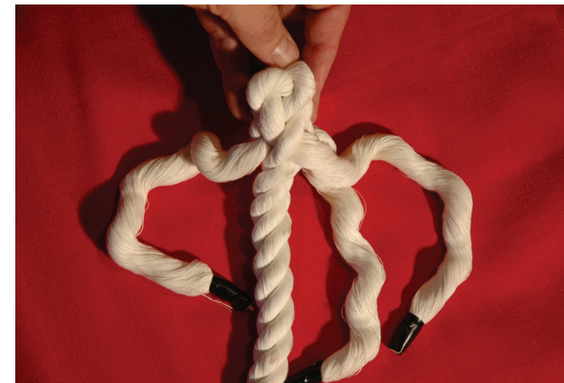
13. This is what the rope should look like after each of the three tails has been back plaited through the rope once. Repeat the process until the strands have been back plaited completely. Do not back plait a strand more than once before rotating to the next strand.
