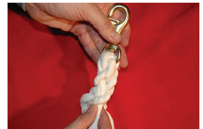
7. Alternate the process with each of the three strands, working down the braided rope. Do the back plaiting process once on each strand, rotating from strand to strand. Do not back plait a strand more than once before moving to the next strand.
