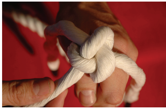
6. Tighten the knot by alternating pulling pressure to each of the strands. This forms a crown knot.
