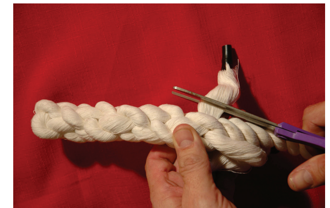
16. The ends can then be cut off. If the plaits are not tight, you may want to tape around the rope in line with the ends of the strands.
