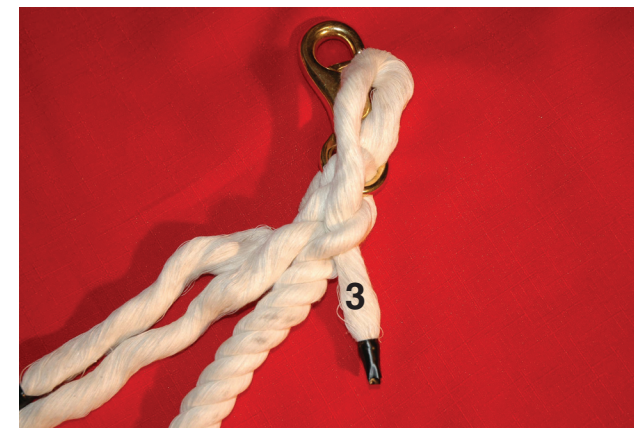
6. The third tail is the strand that was run through the eye the opposite direction of the first two strands. Repeat the same process of plaiting by moving over one strand then under the strand to the right. It may appear that you need to move over two strands before moving under a strand in order for this strand to be aligned evenly with the first two strands.
