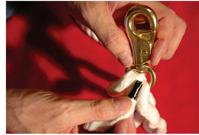
3. Run the remaining strand through the eye in the opposite direction of the first two strands.
