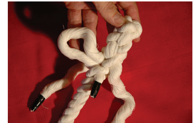
14. The process of rotating each time, and back plaiting over one and then under an underlying strand is repeated until the ends have been back plaited entirely through the underlying, unraveled rope.
