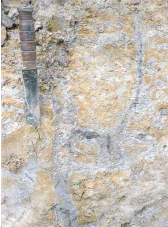
Figure 20. Soil redoximorphic features are used to determine soil zones of water saturation.
