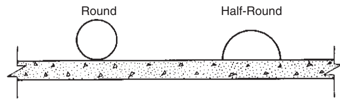
Figure 3. On-floor ducts are usually round or half-round in cross-sections.
