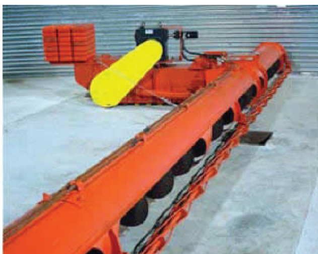
Figure 8. Sweep auger with acceptable guarding.
