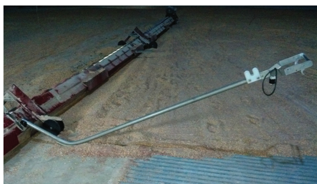
Figure 10. “Dead man” control handle for sweep auger.
