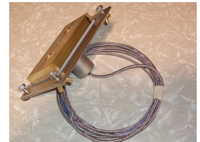
Figure 5: Belt "rub" block to detect belt misalignment.
