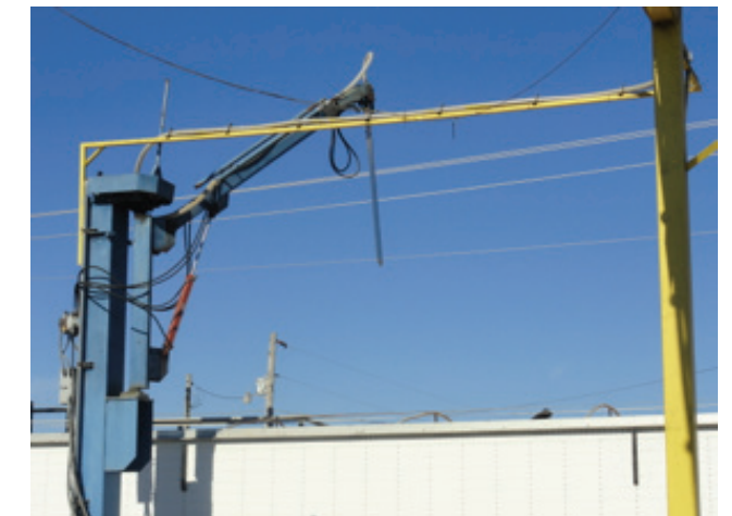
Figure 1. Automatic sampler ready to gather a sample from an incoming grain truck.
