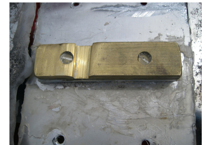
Figure 6: Worn belt alignment block.
