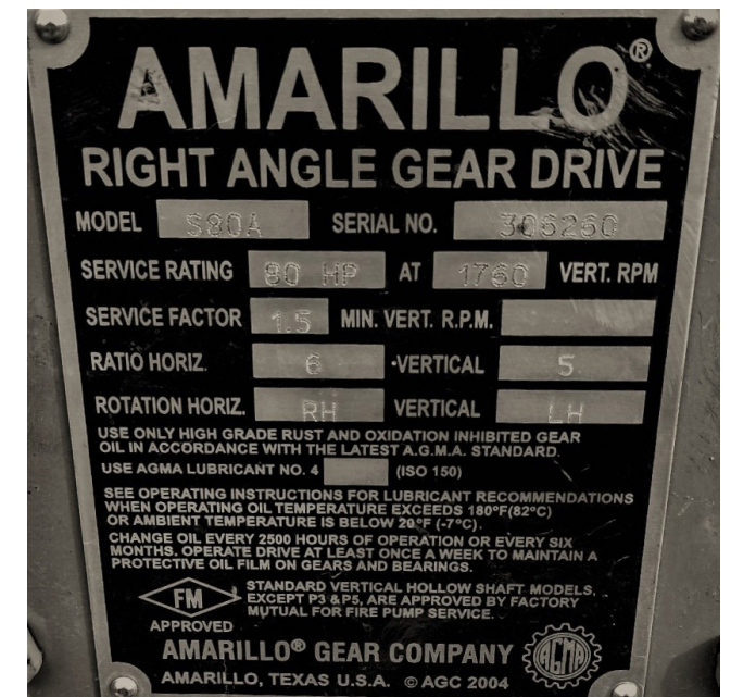
Figure 5. A gear drive nameplate.
