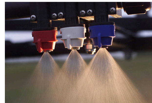
Figure 1. Calibration is the process of adjusting spray equipment to uniformly apply the desired rate of chemical.
