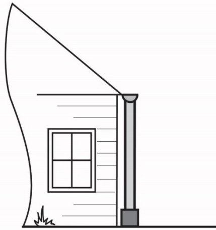
Figure 2. Downspout connected under the ground surface.
