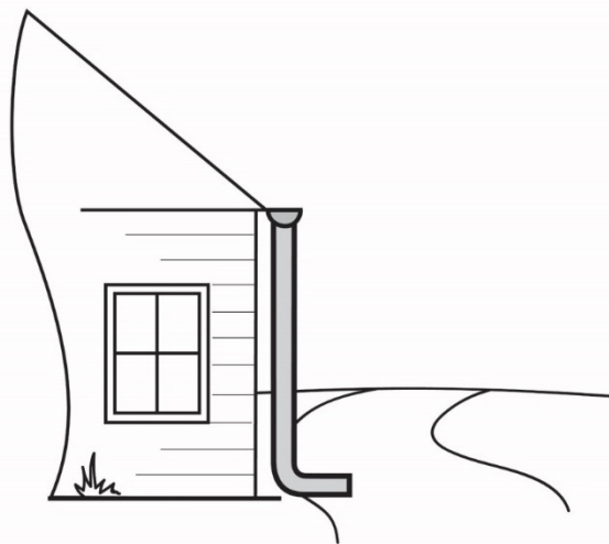
Figure 3. Downspout discharges on driveway.
