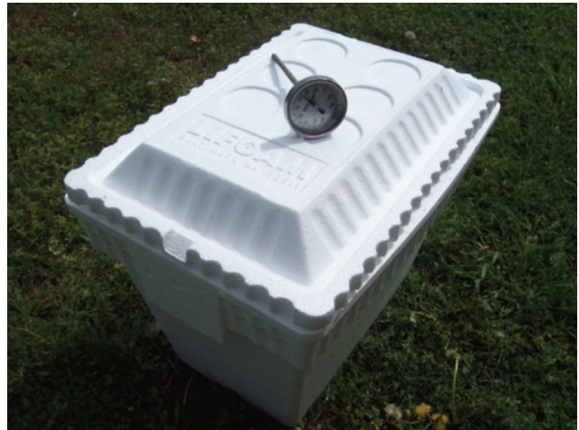
Figure 1. Suitable Styrofoam Cooler and Compost Thermometer for the Icebox test.
