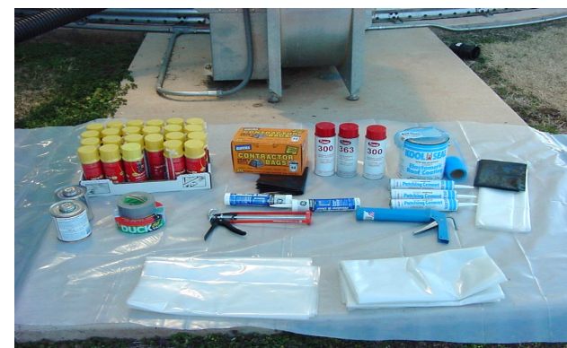
Figure 3. Products used for sealing grain structures. (Photo: Ron Noyes)
