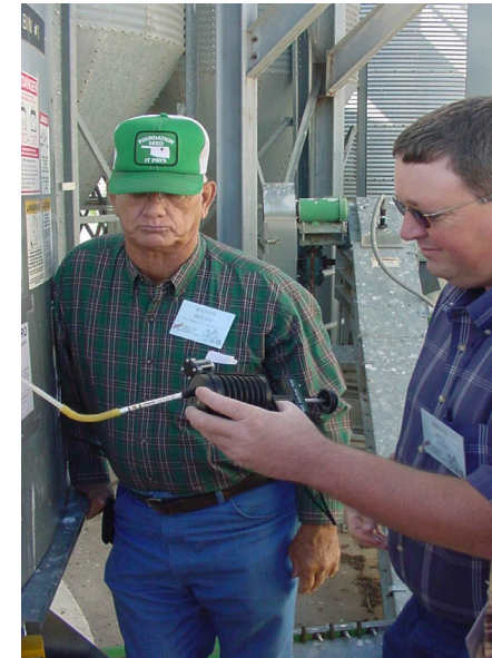
Figure 8. Using gas detection tubes to monitor phosphine levels. (Photo: Edmond Bonjour)
