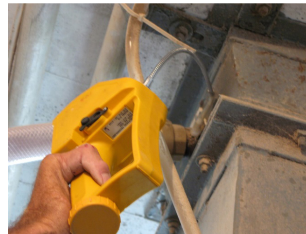
Figure 9. Using an electronic gas detection monitor to determine the level of phosphine gas. (Photo: Edmond Bonjour)
