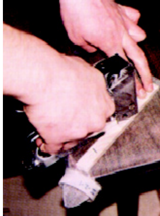
Figure 6F. Staple larger wood lath to inside of cone.
