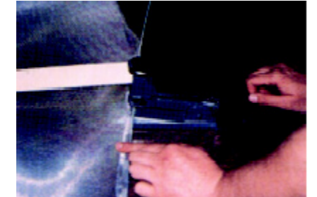
Figure 9F. Staple 9- to 10-gauge wire into fold on shorter side using no. 13 book-binding staples.
