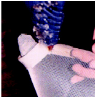
Figure 6D. Attach ring using hot glue.
