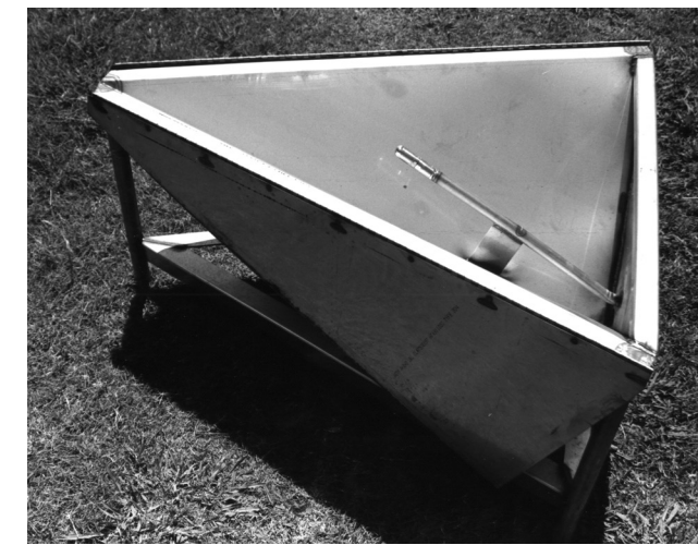
Figure 3. Inclined stainless steel pressure rinse/drain rack.
