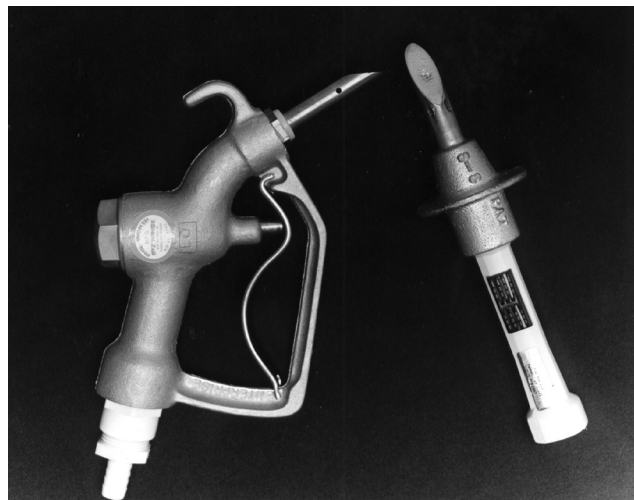
Figure 1. Rinse nozzles used for penetrating plastic or metal containers.
