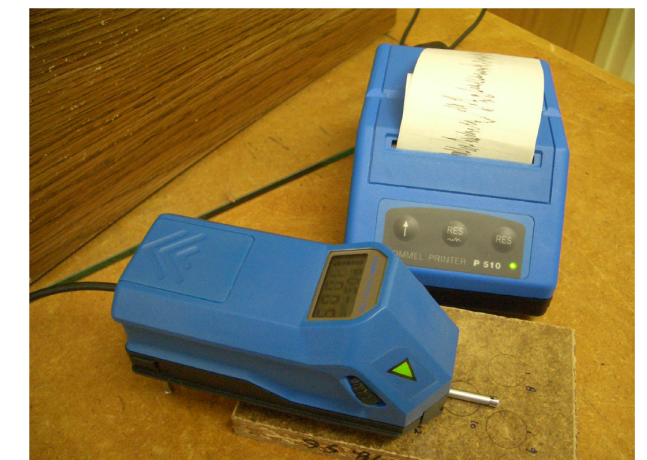
Figure 6. Stylus-type profilometer used in this work.
