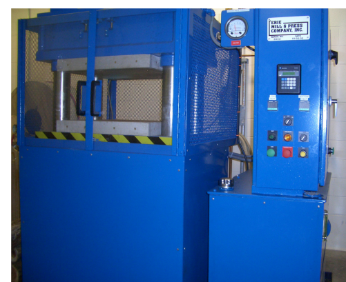
Figure 4. Computer controlled 200 ton hot press.
