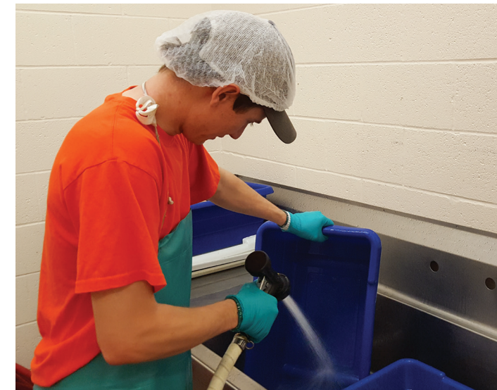
Using a water hose in a food-processing facility. A lower-pressure, lower-flow system that is lighter and easier to operate would save water, energy and reduce splashing. An automated wash system for containers would save on labor, water and energy costs.
