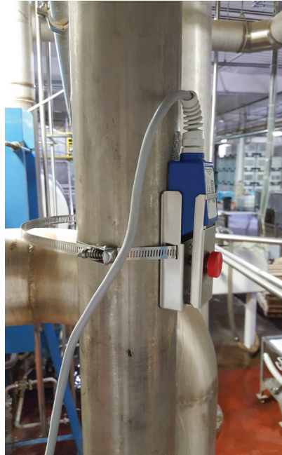
Clamp-on ultrasonic flow sensor (model PDFM 5.1, Greyline Instruments, Inc, Massena, NY) used to accurately measure liquid flow in pipes.
