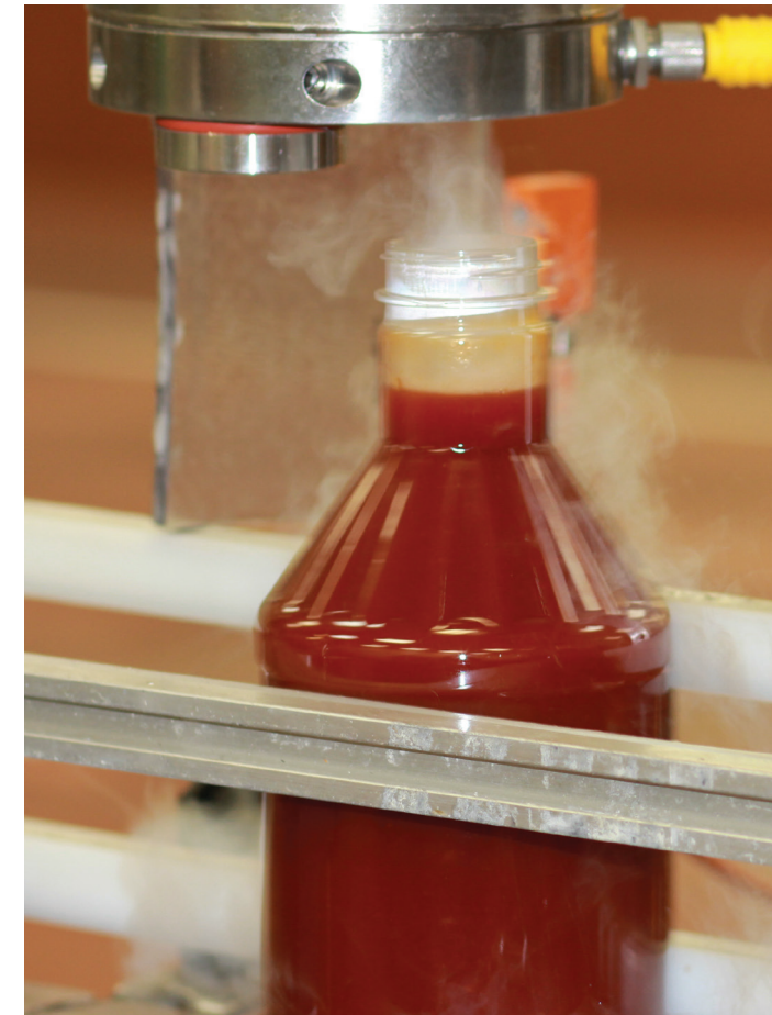
Nitrogen gas used as a processing aid in a barbecue sauce plant.
