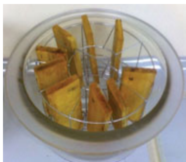
Figure 1. Desiccator formaldehyde emission test setup.
