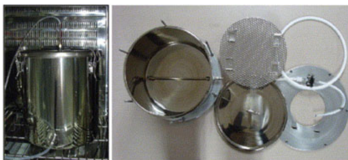
Figure 2. Chamber formaldehyde emission test setup.
