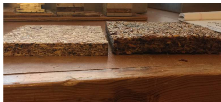
Figure 3. Dry and 24-h water soaked samples.
