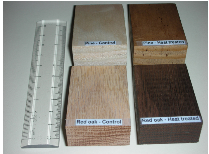
Figure 1. Discoloration of heat-treated samples.
