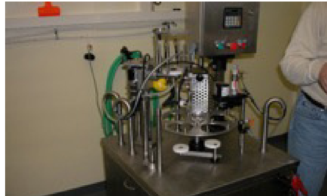
Figure 2. Pump rotary filler for dairy products.
