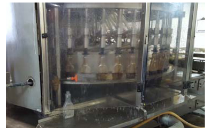
Figure 1. Gravity overflow rotary filler for syrup.
