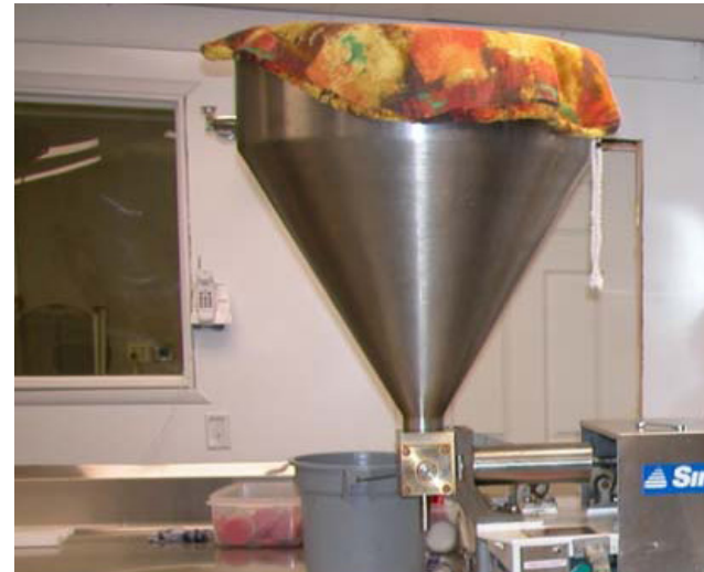
Figure 3. Piston filler with manual container handling.
