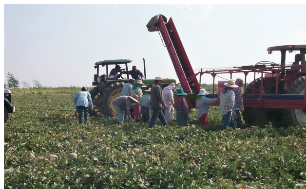
Harvest conveyer to assist hand harvesting.
