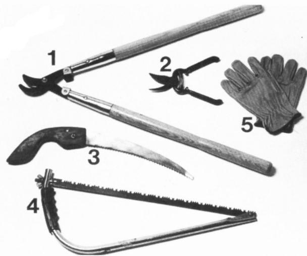
Figure 1. (1) lopping shear (2) hand pruner (3) folding saw for tight places (4) bow saw for limbs and (5) leather gloves. Note, carpenters saws gum up, pruning saws do not.
