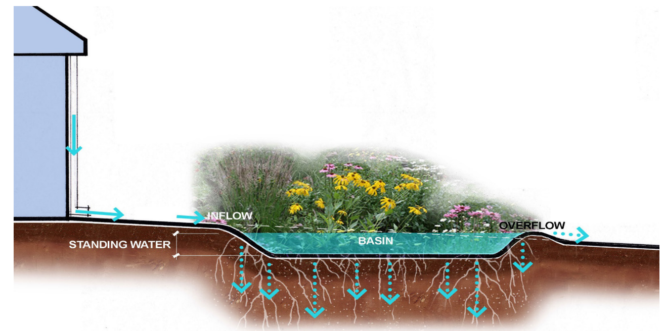
Figure 1. A typical rain garden section with three components: Inflow, Basin and Overflow.
