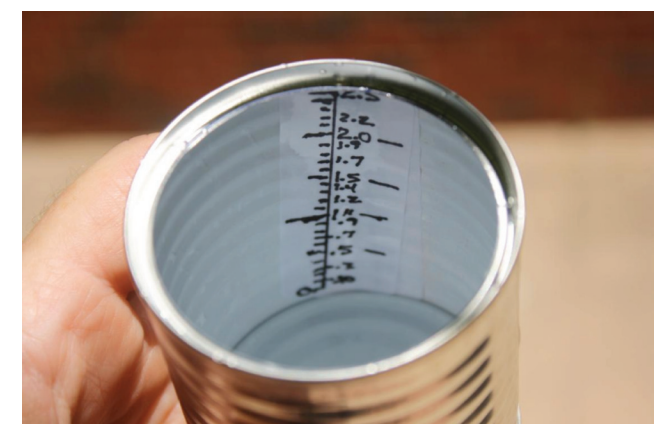
Figure 2. Examples of various catch cups that can be used to conduct the simple irrigation audit and examples of how to mark the side of the catch cups for more accurate irrigation output measurement.
