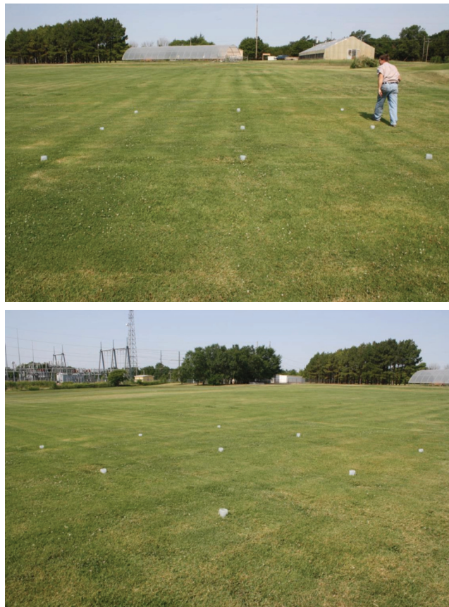
Figure 3. Examples of how to layout the irrigation catch cups in a grid pattern with each cup located about three steps apart from each other.
