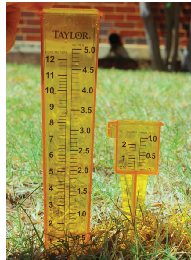
Figure 1. Examples of a short rain gauge (right) that can be used to conduct the simple irrigation audit procedure and a tall rain gauge (left) that should not be used to conduct the simple irrigation audit procedure.
