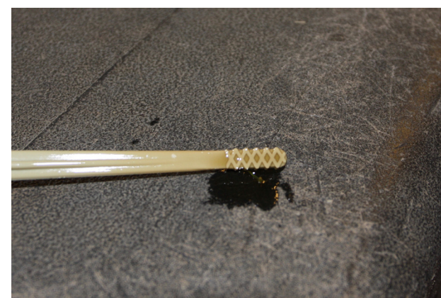
Figure 7. A dipstick's maximum (left arrow) and minimum (right arrow) oil levels.
