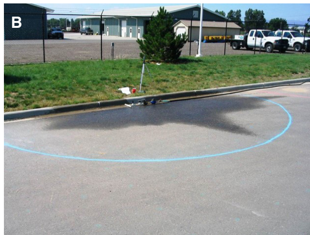
Figures 4a and 4b. At an optimum pressure of 30 psi (top) the spray pattern is evenly distributed. When the pressure is increased to 50 psi (bottom) the spray pattern degrades while the flow rate increases. Photos courtesy of Brent Mecham, Irrigation Association.
