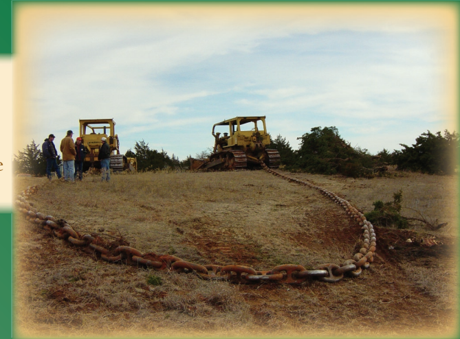
Ground anchor chains make quick work of large eastern redcedar, but are very expensive.
