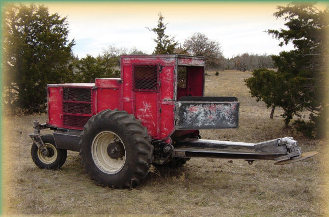
Hydraulic saws work well and are very fast on medium- to large-size trees. They do a good job following a prescribed fire.
