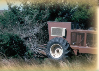
Hydraulic saws work well and are very fast on medium- to large-size trees. They do a good job following a prescribed fire.
