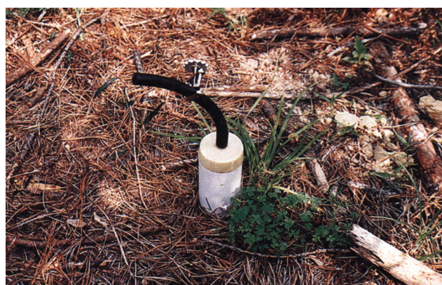
Two Lysimeters were located in each plot and soil water was collected after each significant rainfall.
