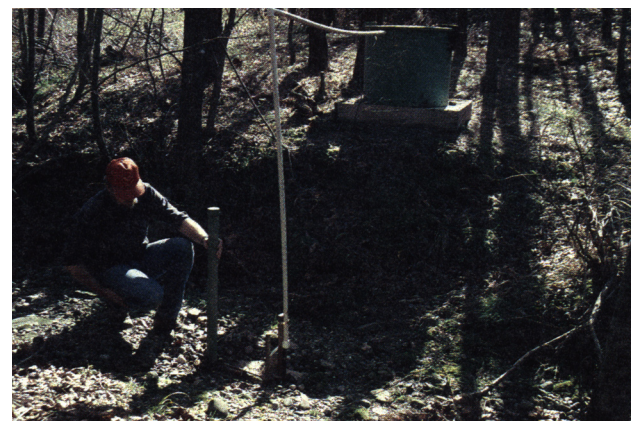
The monitoring sites were located in an intermittent stream channel. The downstream location is shown here. Water samples were automatically collected during stormflow events.
