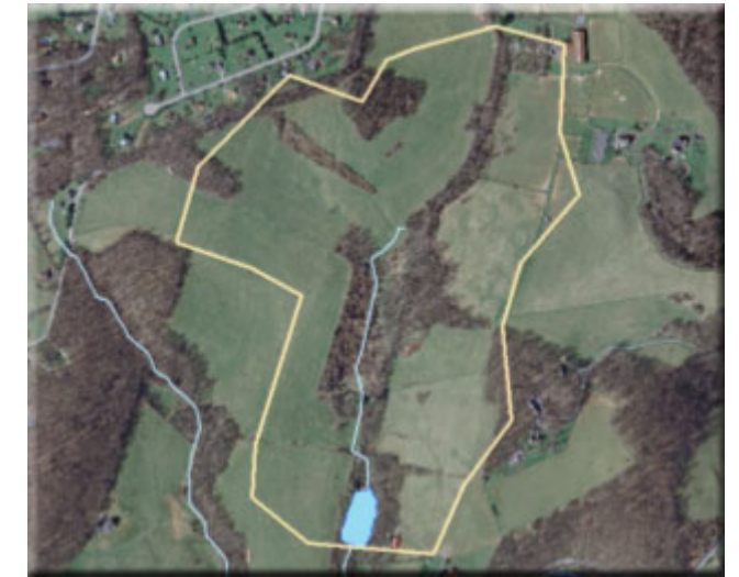
Figure 7. The area of land that slopes towards the pond is known as the watershed. Get to know the boundaries of your pond watershed so you are aware of any problems that might harm the pond. (Credit: Winfield Fairchild, Ponds of Chester County, Pennsylvania)
