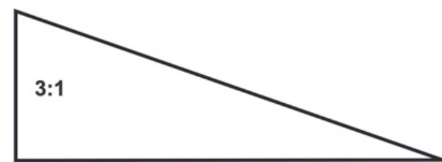
Figure 11. A generally advantageous slope for dam faces and shorelines is 3 feet of “run” for every 1 foot of “rise” (3:1). This reduces erosion potential, decreases the chances of child drownings and makes it possible to mow dam faces to eliminate young trees. Image courtesy Alabama Cooperative Extension Service.
