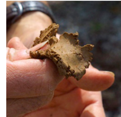
Figure 7. Soil quality matters immensely. The ribbon test is a quick, on-site test for adequate clay content. Not all high clay content soils are suitable for dams - ideally a mixture of clay, sand and silt is needed to allow for good compaction.
