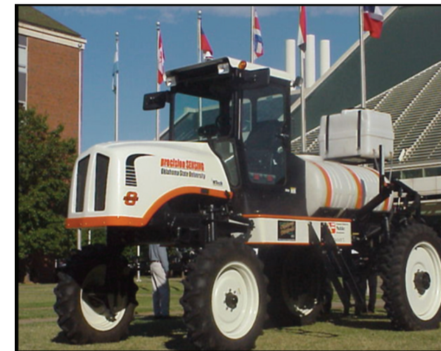
Figure 6. The Cherokee VRT applicator, this sprayer has a 60 ft boom with sensors mounted every 2 ft along the boom.
