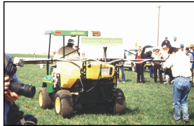
Figure 4. The first demonstration of sensor-based variable N application, Hennessey, OK., 1996
