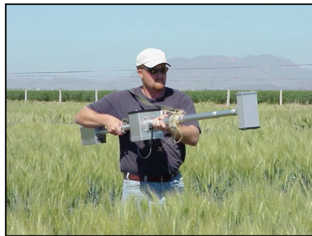
Figure 3. Passive sensor measuring reflectance in spring wheat, Ciudad Obregon MX.
