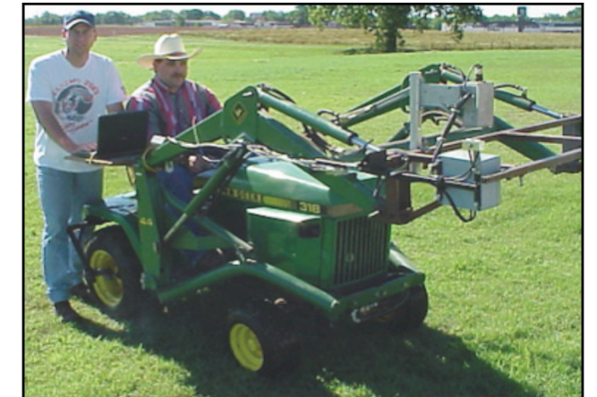
Figure 1. NDVI sensor readings being collected on bermudagrass, Stillwater, OK, 1997.
