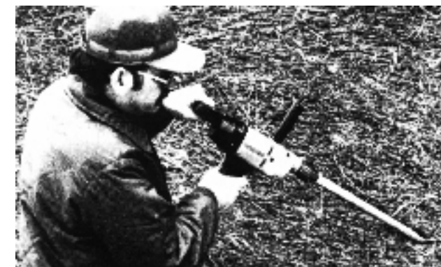
Figure 1. Forage probe mounted on an electric drill.
