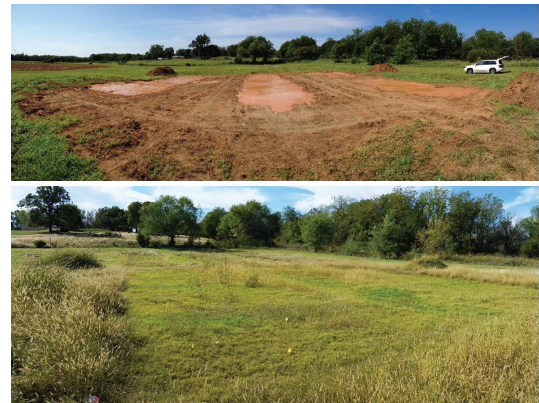
Figure 4. Scraped/bare soil plots pictured immediately after surface application (upper) and approximately 120 days after application (lower).
