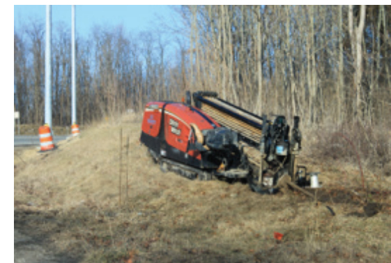
Figure 1. Picture of a HDD rig, and a schematic showing the non-invasive, trenchless technology that HDD rigs provide.
