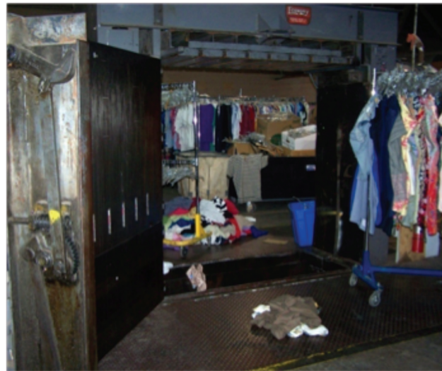
Figure 1. A steel baler with a deep pit compacts unwanted textiles into bales.
