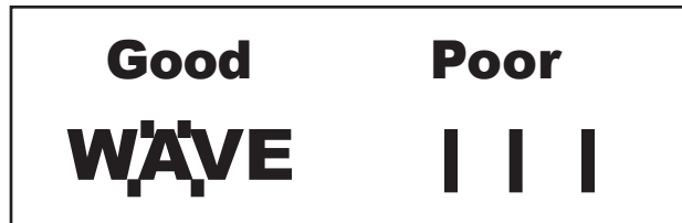
Figure 4. When using stencils or rub-off lettering, make sure letters are spaced properly. Allow for the shape of the letters
